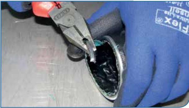
5. Bend the metal clip profile forward at a 90° angle to the hose.
