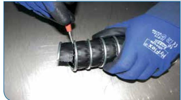
3. Peel the end of the metal helix, so that it is free from the wall material. Remove the material with a sharp instrument. Please ensure that you cut away from your body, in order to avoid any injuries.
