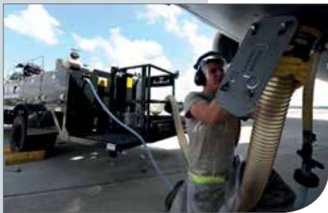
TSU - (Toilet Service Unit)
