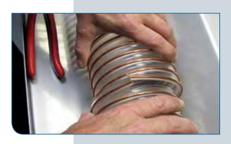
Finally, cut off the hose material cleanly along the reinforcement spiral.
