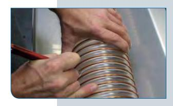
Pull both ends of the hose apart and cut the reinforcement helix using wire cutters.
