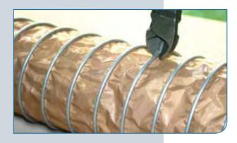
Using a sharp knife, cut the hose material through to both adjacent helixes.
