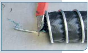
6. Remove any remaining material from the metal clip profile.
