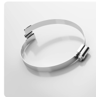
Car-Grip Hose Clamp, screwable, Steel quality W4, stainless steel 1.4301 special clamp for attaching Carflex Super and Master-PUR STEP hoses to mobile and stationary systems
