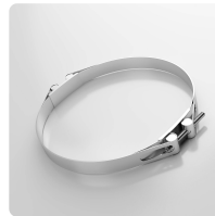
Hose Clamp with Bolts, Steel quality W4, stainless steel 1.4301 Special clamp for fastening medium and heavy spiral hoses to connection pipes on mobile and stationary units
